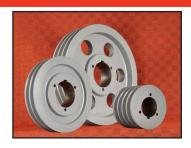
Where the application demands are rugged, and torques and shafts sizes dictate flexibility in mounting our classic and **Heavy Duty Sheaves** meet the task. Heavy Duty cast iron sheaves available **QD**, **TB Taper Bushed**, or **DST-Double Split Taper** designs. They can accept A/B, C, 3V, 5V, and 8 V belts. One thru 12 groove configurations with outside diameters of 2.2-71" cover the gambit. Naturally, we stock all of the Bushing types for mounting of the Sheave options. Have it Your Way!
